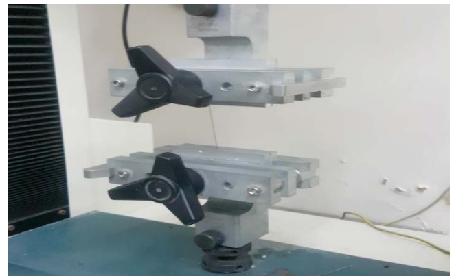
Figure 2: The ends of the wire were attached to the fixtures of the universal testing machine
