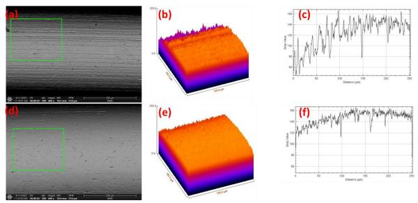
Figure (8): SEM and image analysis results of the for control (a, b, and c) and intervention (d, e, and f) groups. The SEM results at magnification 400X (a and d), the surface plot (b and d), plot profile (c and f).
