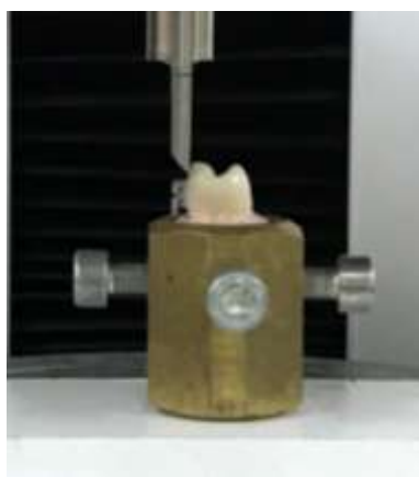
Fig 3: Position of the tapered blade in relation to the tooth
